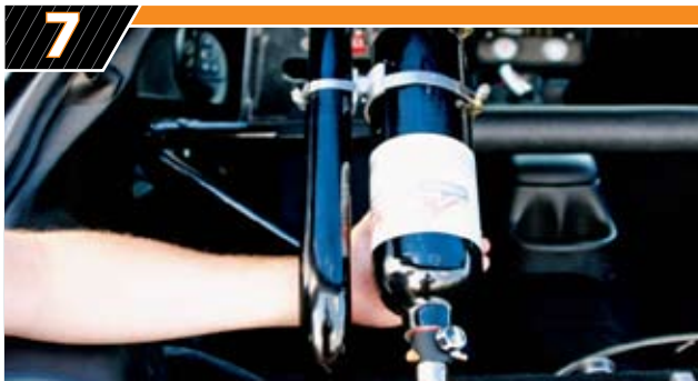
After verifying the 12-inch supply line would reach the nitrous bottle, the NANO bottle is centered in the mounting brackets.
