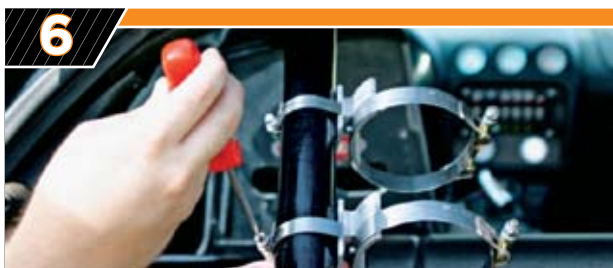
The NANO cylinder can be mounted "piggyback" onto your existing nitrous bottle or anywhere within the range of the 12-inch hose. Since the '02 TA's nitrous bottle was equipped with a Wolfe Racecraft 10-point rollcage, the driver-side tube proved to be the perfect place to mount the two supplied brackets.
