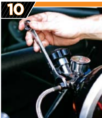
While the NANO regulator is turned off, the 12-inch supply line is fitted to the nitrous bottle with an 11/16-inch wrench. In addition to pressurizing the system once the valve is opened, it should be noted that the NANO system contains an anti-reversion valve at this connection. In layman's terms, you won't lose precious nitrous or HPA when disconnecting the nitrous bottle in order to refill it.
