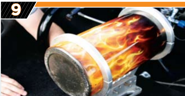
Equipped with an Aerospace Components billet nitrous bottle bracket, the owner slips the bottle into the bracket and inserts the mounting pins.
