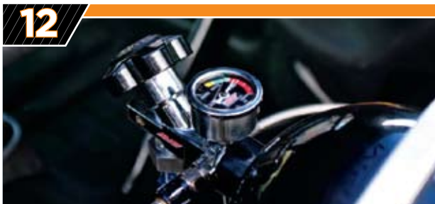
Once the system was hooked up and all the fittings were double-checked to be tight, the NANO bottle and the nitrous bottle valves were opened. After verifying that no leaks existed, the NANO-supplied liquid-filled bottle pressure gauge showed 1,150 psi.
