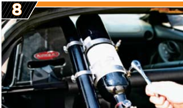
A 1/2-inch socket secures the bottle.
