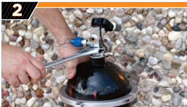
The NANO kit fits any approved 10-pound nitrous bottle, and for an additional $35 you can upgrade to a kit designed for 15-pound bottles. Installing the kit begins by removing the siphon tube from the nitrous bottle. After ensuring the contents of the nitrous bottle are empty, remove the old siphon tube with an adjustable wrench and secure the NANO tube to the nitrous bottle.
