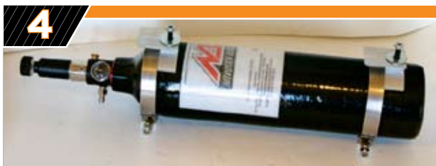
Once complete, get out the NANO cylinder, which is equipped with a Nitrous Pressure Compensator that features an On/Off knob and a 6,000-psi pressure gauge. Direct from NANO, the cylinder was full of high-pressure air (HPA) and was set to 4,500 psi. Although high-pressure nitrogen (HPN) may be used, NANO recommends HPA, as it is readily available and typically $3-$5 at most paintball and scuba shops. In addition, if you are pals with any firefighters, inquire about the SCBA re-fillers common at almost any fire station across the country.
