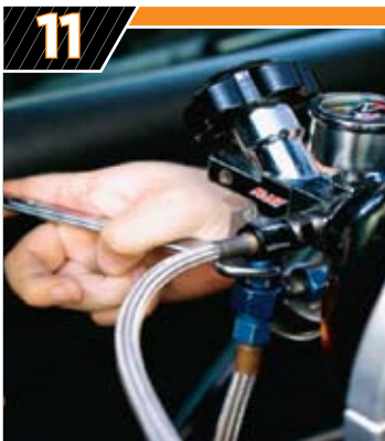
The nitrous line that feeds the engine is then screwed onto the bottle nipple and tightened. The universal kit utilizes a modified NOS SuperHiFlo valve that will sustain a flow rate of 0.45 pounds of nitrous oxide per second. According to Darnell, "This typically takes care of up to 550 hp (a 550 shot), and for even greater nitrous flow, our Evil-Twin kit will flow .70 pounds per second, good for roughly 850 hp."
