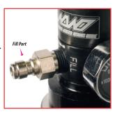
Always evacuate excess air/nitrogen from the nitrous oxide bottle before doing a nitrous refill by turning the nitrous bottle side down, gently opening the nitrous valve, and letting pressure flow from the bottle until you see vapor escape from the bottle valve. Then shut the valve off and fill the nitrous bottle in the customary manner.
