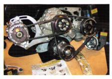
Jones Racing Products' [(610) 847-2028; www.jonesracingproducts.com] PRI display. The billet-aluminum brackets are lightweight, and the alternator bracket is perfect for the 5.0 racer who wants to run his 'Stang with an alternator without the bulk and weight of the factory bracket. The bracket holds a 130A, 3G alternator with no problem.
